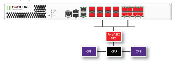
You can use the following get command to display the FortiGate 400D NP6 configuration. The command output shows one NP6 named NP6\_0 and the interfaces (ports) connected to it. You can also use the diagnose npu np6 portlist command to display this information.
