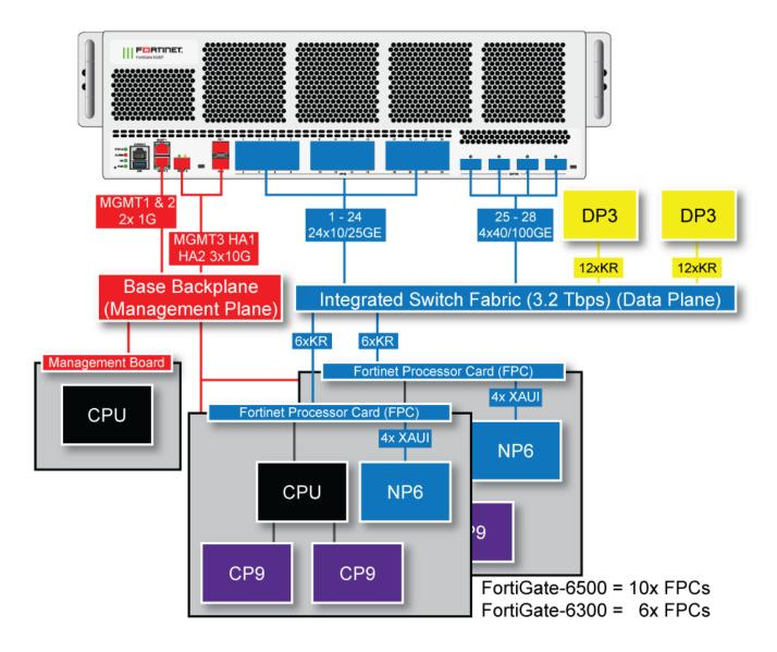
In the data plane, two DP3 load balancers use session-aware load balancing to distribute sessions from the front panel interfaces (port1 to 28) to Fortinet Processor Cards (FPCs). The DP3 processors communicate with the FPCs across the 3.2Tbps integrated switch fabric. Each FPC processes sessions load balanced to it. The FPCs send outgoing sessions back to the integrated switch fabric and then out the network interfaces to their destinations.
