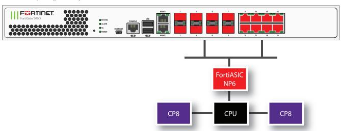
You can use the following get command to display the FortiGate 500D NP6 configuration. The command output shows one NP6 named NP6\_0 and the interfaces (ports) connected to it. You can also use the diagnose <code>npu np6 portlist</code> command to display this information.
