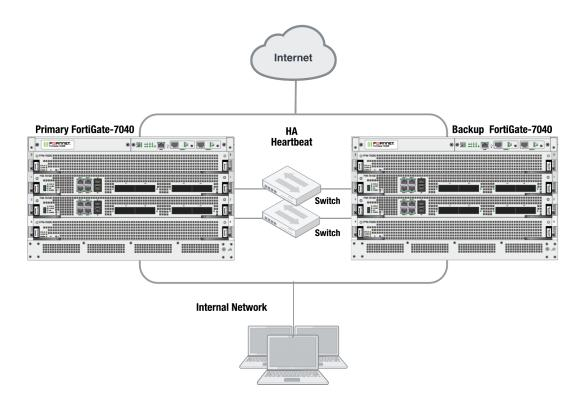
The primary FortiGate-7000 processes all traffic. The backup FortiGate-7000 operates in hot standby mode. The FGCP synchronizes the configuration, active sessions, routing information, and so on to the backup FortiGate-7000. If the primary FortiGate-7000 fails, traffic automatically fails over to the backup FortiGate-7000.
