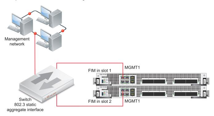
The following example shows redundant connections between both FIMs and the switch. In this case you need to add more switch ports to the static aggregate interface on the switch. You do not have to change the configuration of the FortiGate-7000 to set up this redundant management connection configuration.
