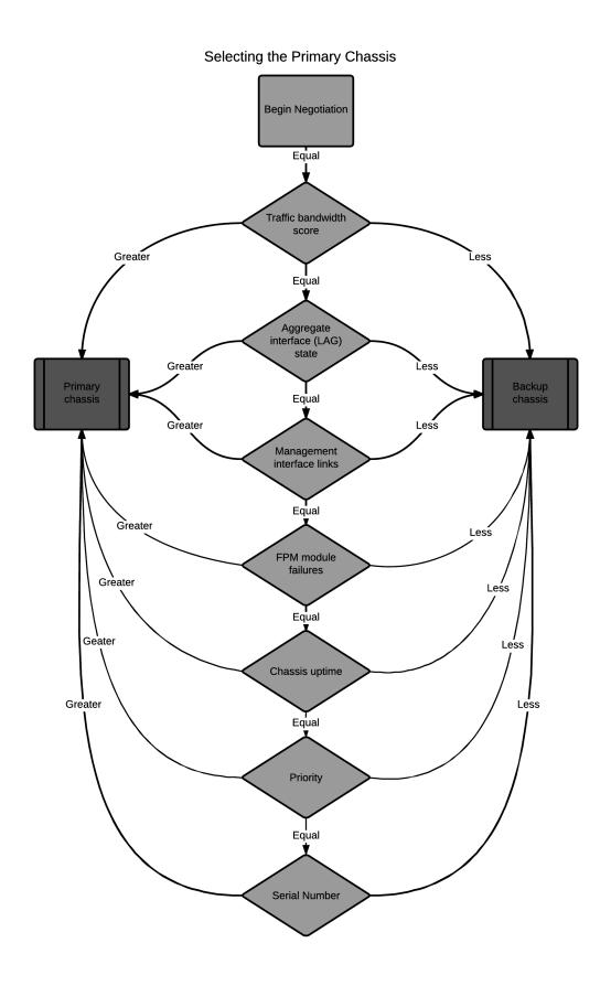
If there are no failures and if you haven't configured any settings to influence primary chassis selection, the chassis with the highest serial number to becomes the primary chassis.
