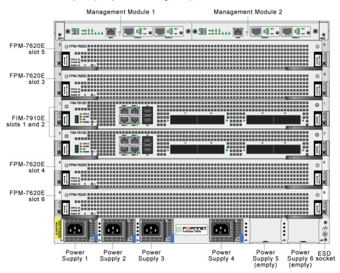
Power is provided to the chassis using four hot swappable 3+1 redundant 100-240 VAC, 50-60 Hz power supply units (PSUs). You can also optionally add up to six PSUs to provide 3+3 redundancy. The FortiGate-7060E can also be equipped with DC PSUs allowing you to connect the chassis to -48V DC power
