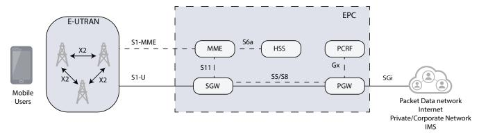
FortiOS Carrier can be installed in any of the GTP data streams in your network, depending on the type of protection that you need. For overall protection you can install FortiOS Carrier between the mobile users and the EPC. If you are concerned about protecting the EPC from the internet or about protecting packet data networks, you can install FortiOS Carrier between the EPC and any TCP/IP networks that the EPC connects to.
