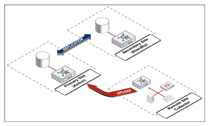
Under normal operations, if collectors are being used, these upload to Site 1, the Primary site, and will buffer by design when this site is not available. If DR is set up and a disaster occurs, then these same collectors will revert to uploading to Site 2, the Secondary site, which will now be designated as the Primary/Active site.
