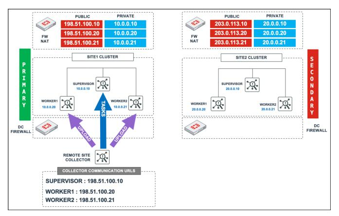
At this point, the Primary node (Site 1) is unavailable. The remote Collector nodes are essentially hard-coded (by IP) to talk to the Primary site only. Even if Site 2 (the Secondary node) is up and operational and promoted to be the Primary node, Collectors are unable to upload logs or get any tasks from the Supervisor node due to the old Primary sites IPs being used.
