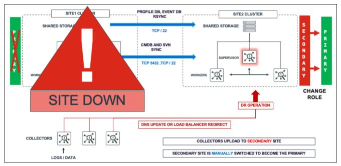
When the Old Primary (Site 1) is recovered and powered up, it will sync missing data with the Secondary site (Site 2, the Active Primary FortiSIEM) once it is added back as a new Secondary site.
