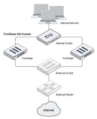
FGCP HA provides a solution for two key requirements of critical enterprise networking: enhanced reliability and increased performance, through device, link, and remote link failover protection. Extended FGCP features include full mesh HA and virtual clustering. You can also fine tune the performance of the FGCP to change how a cluster forms and shares information among cluster units and how the cluster responds to failures.
