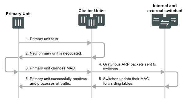
When a cluster starts up, after a failover, the primary unit sends gratuitous ARP packets to update the switches connected to the cluster interfaces with the virtual MAC address. The switches update their MAC forwarding tables with this MAC address. As a result, the switches direct all network traffic to the primary unit. Depending on the cluster
