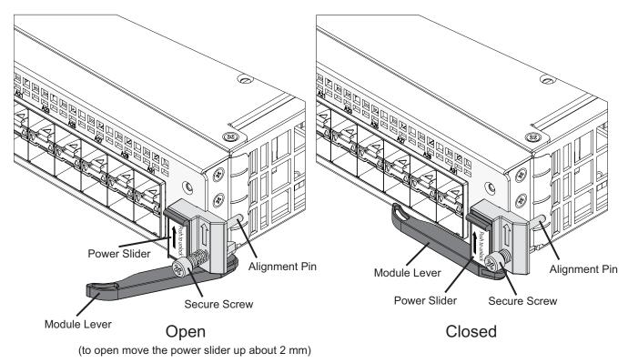
The FIM-7901E module levers align the module in the chassis slot and insert and eject the module from the slot. The power sliders activate micro switches that turn on or turn off power to the module. When both sliders are raised, the module cannot receive power. When the sliders are fully closed, the module can receive power if it is fully inserted into a chassis slot.
