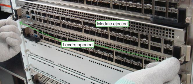
6. Hold the levers to slide the module part way out of the chassis slot. Then grasp the module by the sides and carefully slide it out of the slot.
