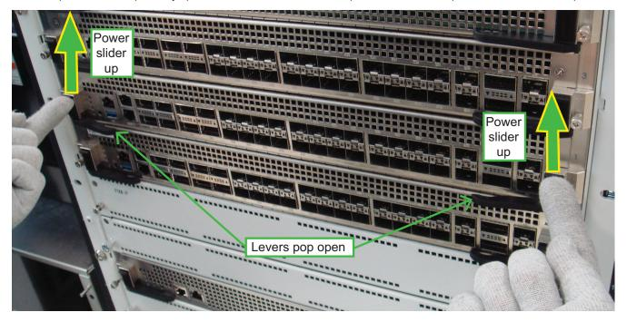
5. Use moderate force to fully open the levers and eject the module from the chassis.
