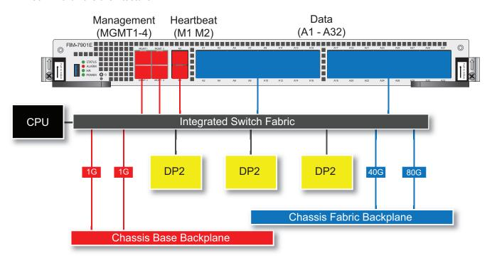
This chapter describes installing a FIM-7901E interface module into a FortiGate-7000 chassis.
