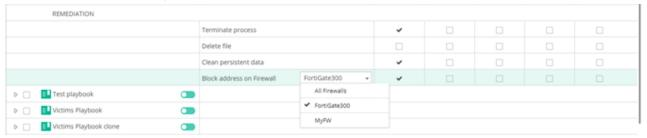
FortiEDR is now configured to add malicious IP addresses to the blocking policy on the firewall upon triggering of a security event. You can check that malicious IP addresses are added to the address group that was configured in FortiGate following FortiEDR security events.
