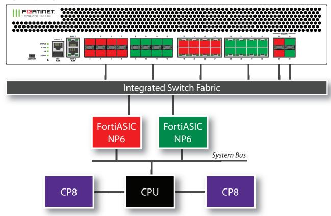
You can use the following get command to display the FortiGate 1200D NP6 configuration. The command output shows two NP6s named NP6 $_0$  and NP6 $_1$ . The output also shows the interfaces (ports) connected to each NP6. You can also use the <code>diagnose npu np6 port-list</code> command to display this information.
