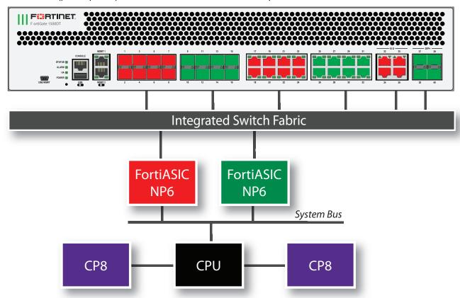
You can use the following get command to display the FortiGate 1500DT NP6 configuration. The command output shows two NP6s named NP6\_0 and NP6\_1. The output also shows the interfaces (ports) connected to each NP6. You can also use the diagnose <code>npu np6 port-list</code> command to display this information.
