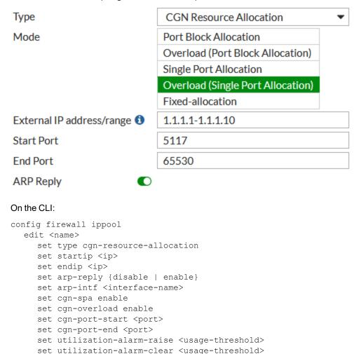
An overload single port allocation CGN resource allocation IP pool assigns single ports instead of ranges of ports. This type of CGN IP pool conserves ports by effectively reducing the port block size to 1. Since this is an overload IP pool, ports are re-used. A client session can get any port from the range of ports added to the IP pool that are available.
