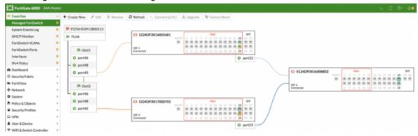
**5.** Finalize by doubling the ICL links between the two distribution switches.
