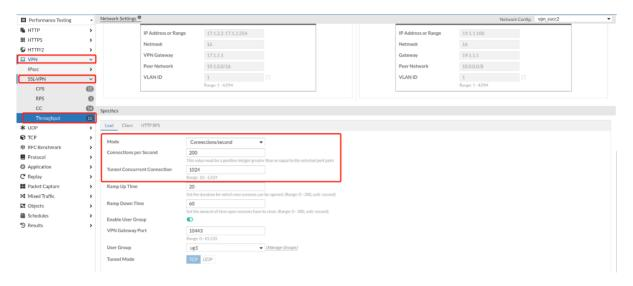
The "Tunnel Concurrent Connection" item is the total number of tunnels created in the Throughput case.
