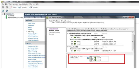
3. For VLAN ID, select All (4095), if you are using Trunk port on the switch. Click Next and then Finish to complete the vSwitch creation.
