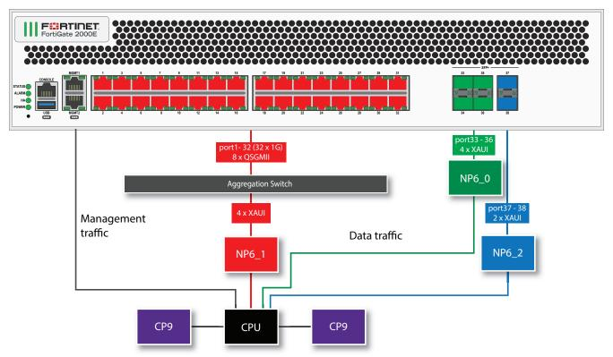
All data traffic passes from the data interfaces to the NP6 processors. Data traffic processed by the CPU takes a dedicated data path through the ISF and an NP6 processor to the CPU.
