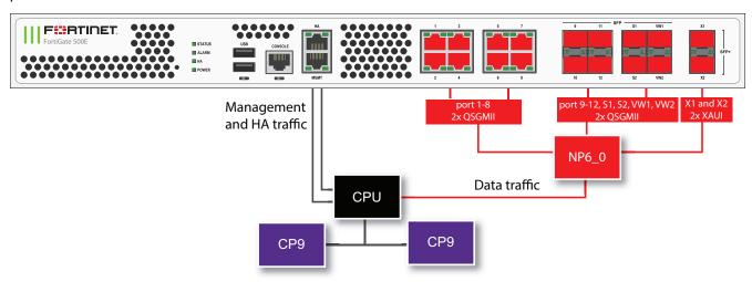
The FortiGate 500E and 501E each include one NP6 processor. All supported traffic passing between any two data interfaces can be offloaded by the NP6 processor. Data traffic to be processed by the CPU takes a dedicated data path through the NP6 processor to the CPU.
