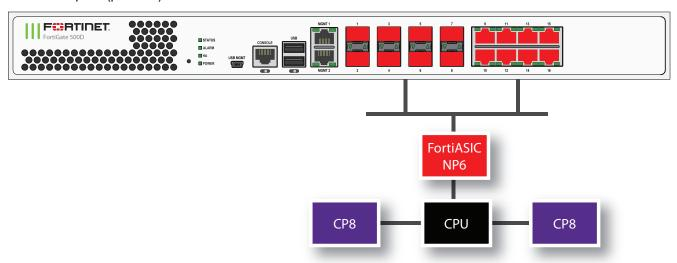
You can use the following get command to display the FortiGate 500D NP6 configuration. The command output shows one NP6 named NP6\_0 and the interfaces (ports) connected to it. You can also use the  $diagnose\ npu\ np6\ portlist$  command to display this information.
