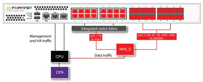
The FortiGate 300E and 301E each include one NP6 processor. All supported traffic passing between any two data interfaces can be offloaded by the NP6 processor. Data traffic to be processed by the CPU takes a dedicated data path through the NP6 processor to the CPU. Interfaces 1 to 16 connect to an integrated switch fabric to allow these sixteen interfaces to share two XAUI ports that connect to the NP6 processor.
