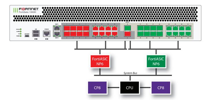
You can use the following get command to display the FortiGate 1000D NP6 configuration. The command output shows two NP6s named NP6\_0 and NP6\_1. The output also shows the interfaces (ports) connected to each NP6. You can also use the diagnose <code>npu np6 port-list</code> command to display this information.
