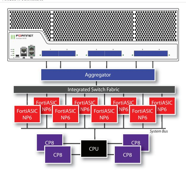
You can use the following get command to display the FortiGate 3810D NP6 configuration. The command output shows all NP6s connected to each interface (port) with cross-chip offloading supported for each port. You can also use the diagnose npu np6 port-list command to display this information.
