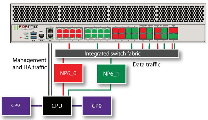
The FortiGate 1100E and 1101E each include two NP6 processors. All front panel data interfaces and both NP6 processors connect to the integrated switch fabric (ISF). All data traffic passes from the data interfaces through the ISF to the NP6 processors. Because of the ISF, all supported traffic passing between any two data interfaces can be offloaded by the NP6 processors. Data traffic processed by the CPU takes a dedicated data path through the ISF and an NP6 processor to the CPU.
