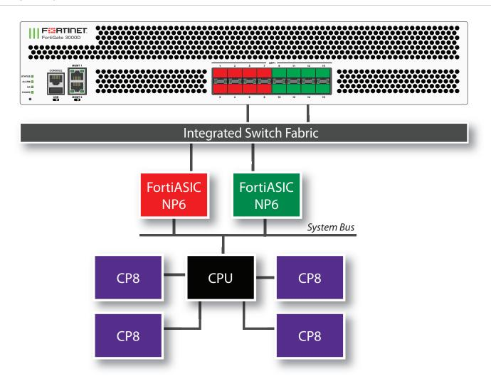
You can use the following get command to display the FortiGate 3000D NP6 configuration. The command output shows two NP6s named NP6\_0 and NP6\_1 and the interfaces (ports) connected to each NP6. You can also use the <code>diagnose npu np6 port-list</code> command to display this information.
