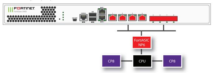
You can use the following get command to display the FortiGate 300D NP6 configuration. The command output shows one NP6 named NP6\_0 and the interfaces (ports) connected to it. You can also use the diagnose <code>npu np6 portlist</code> command to display this information.
