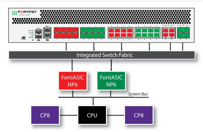
You can use the following get command to display the FortiGate 1500DT NP6 configuration. The command output shows two NP6s named NP6 $\_$ 0 and NP6 $\_$ 1. The output also shows the interfaces (ports) connected to each NP6. You can also use the <code>diagnose npu np6 port-list</code> command to display this information.
