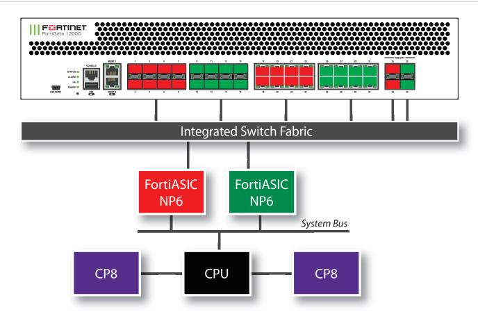
You can use the following get command to display the FortiGate 1200D NP6 configuration. The command output shows two NP6s named NP6\_0 and NP6\_1. The output also shows the interfaces (ports) connected to each NP6. You can also use the diagnose <code>npu np6 port-list</code> command to display this information.
