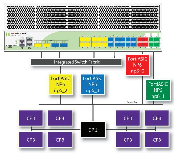
You can use the following get command to display the FortiGate 3700D NP6 configuration. In this output example, the first two NP6s (np6\_0 and np6\_1) are configured for low latency. The command output shows four NP6s named NP6\_0,
