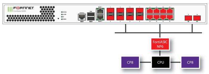
You can use the following get command to display the FortiGate 600D NP6 configuration. The command output shows one NP6 named NP6\_0 and the interfaces (ports) connected to it. You can also use the diagnose <code>npu np6 portlist</code> command to display this information.
