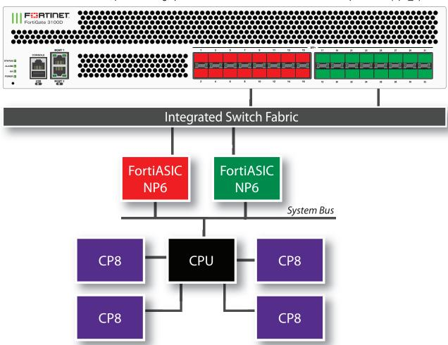
You can use the following get command to display the FortiGate 3100D NP6 configuration. The command output shows two NP6s named NP6\_0 and NP6\_1 and the interfaces (ports) connected to each NP6. You can also use the diagnose npu np6 port-list command to display this information.
