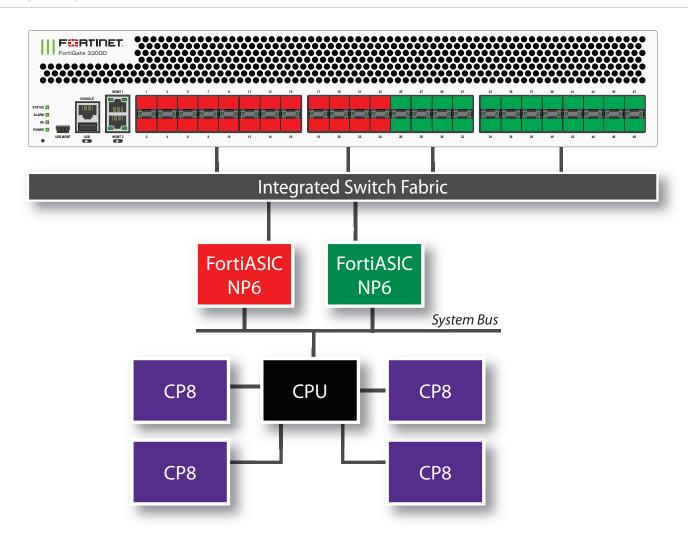
You can use the following get command to display the FortiGate 3200D NP6 configuration. The command output shows two NP6s named NP6\_0 and NP6\_1 and the interfaces (ports) connected to each NP6. You can also use the <code>diagnose npu np6 port-list</code> command to display this information.
