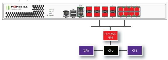
You can use the following get command to display the FortiGate 400D NP6 configuration. The command output shows one NP6 named NP6\_0 and the interfaces (ports) connected to it. You can also use the diagnose <code>npu np6 portlist</code> command to display this information.
