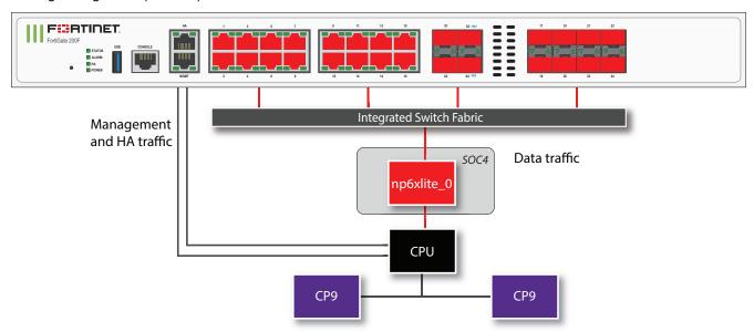
All front panel data interfaces and the NP6XLite processor connect to the integrated switch fabric (ISF). All data traffic passes from the data interfaces through the ISF to the NP6XLite processor. All supported traffic passing between any two data interfaces can be offloaded by the NP6XLite processor. Data traffic to be processed by the CPU takes a dedicated data path through the ISF and the NP6XLite processor to the CPU.
