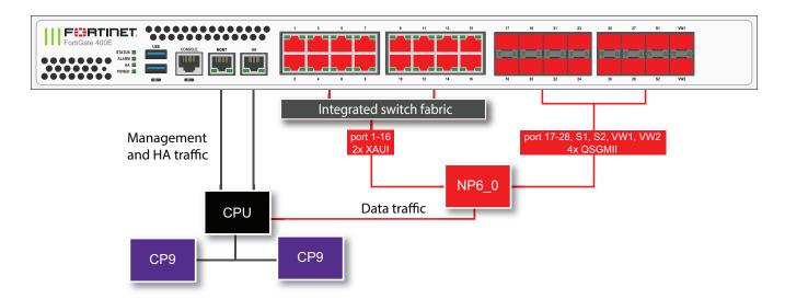
The FortiGate 400E and 401E each include one NP6 processor. All supported traffic passing between any two data interfaces can be offloaded by the NP6 processor. Data traffic to be processed by the CPU takes a dedicated data path through the NP6 processor to the CPU. Interfaces 1 to 16 connect to an integrated switch fabric to allow these sixteen interfaces to share two XAUI ports that connect to the NP6 processor.
