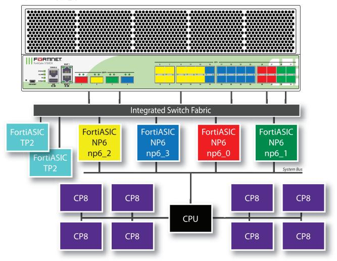
You can use the following get command to display the FortiGate 3700D NP6 configuration with low latency turned off for np6\_0 and np6\_1. The command output shows four NP6s named NP6\_0, NP6\_1, NP6\_2, and NP6\_3 and the interfaces (ports) connected to each NP6. You can also use the diagnose npu np6 port-list command to display this information.
