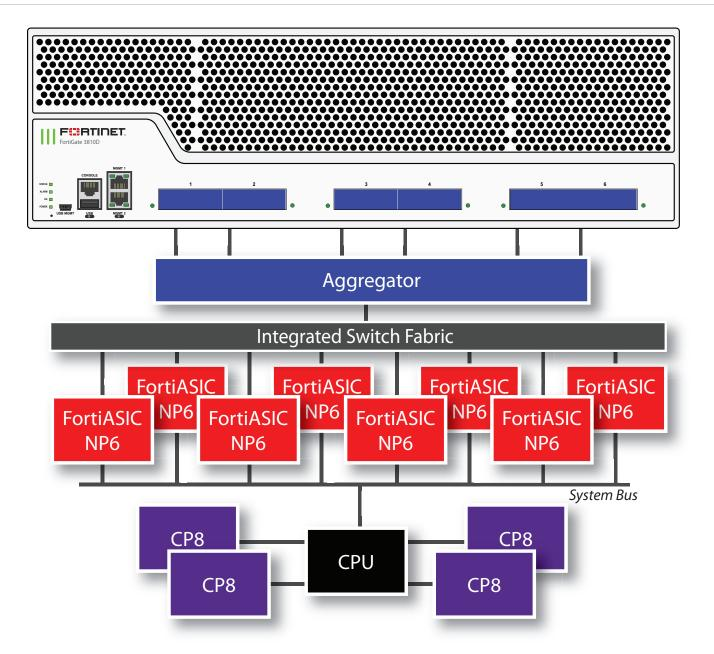
You can use the following get command to display the FortiGate 3810D NP6 configuration. The command output shows all NP6s connected to each interface (port) with cross-chip offloading supported for each port. You can also use the diagnose npu np6 port-list command to display this information.
