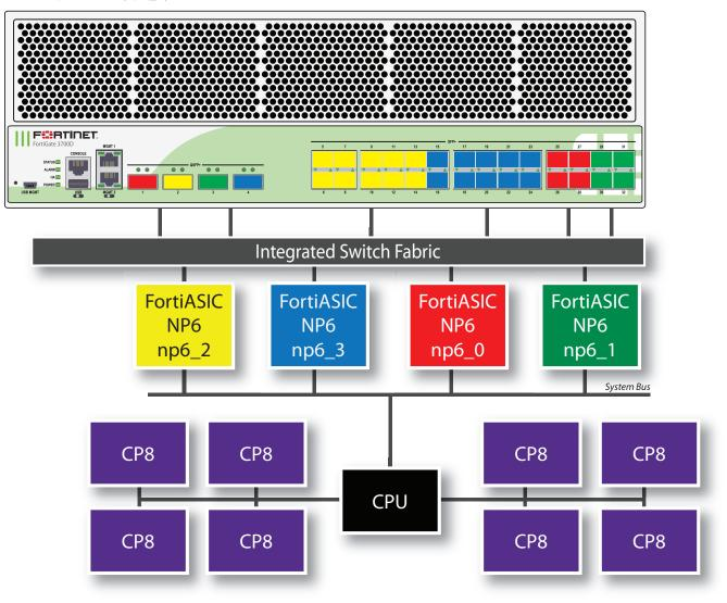
You can use the following get command to display the FortiGate 3700D NP6 configuration with low latency turned off for np6\_0 and np6\_1. The command output shows four NP6s named NP6\_0, NP6\_1, NP6\_2, and NP6\_3 and the interfaces (ports) connected to each NP6. You can also use the diagnose npu np6 port-list command to display this information.
