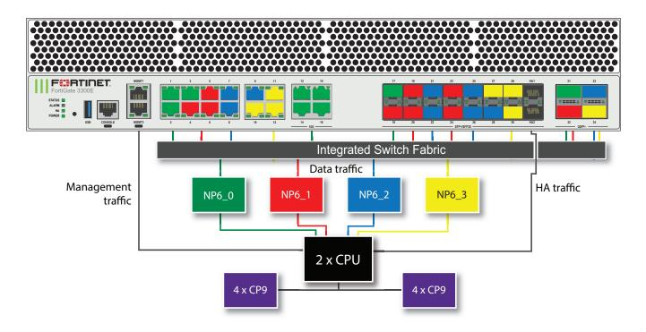
The FortiGate 3300E and 3301E each include four NP6 processors. All front panel data interfaces and all of the NP6 processors connect to the integrated switch fabric (ISF). All data traffic passes from the data interfaces through the ISF to the NP6 processors. Because of the ISF, all supported traffic passing between any two data interfaces can be offloaded by the NP6 processors. Data traffic processed by the CPU takes a dedicated data path through the ISF and an NP6 processor to the CPU.
