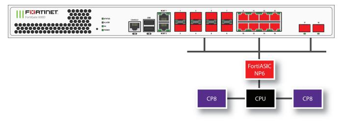
You can use the following get command to display the FortiGate 600D NP6 configuration. The command output shows one NP6 named NP6\_0 and the interfaces (ports) connected to it. You can also use the diagnose npu np6 portlist command to display this information.
