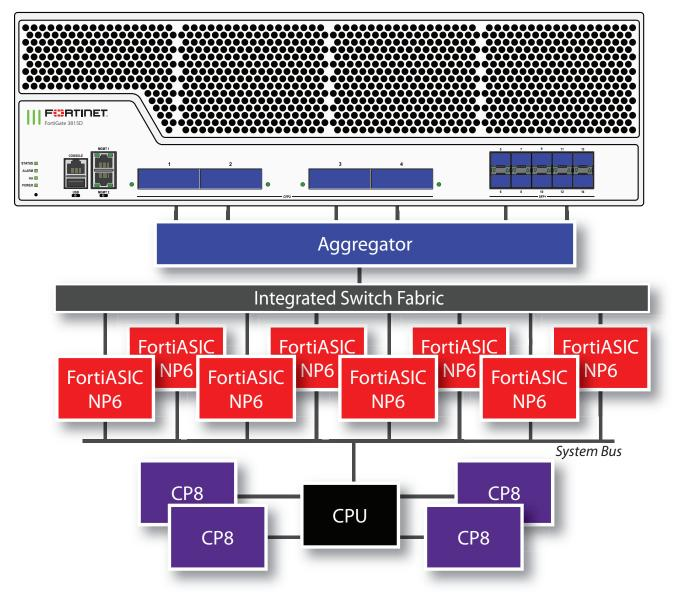
You can use the following get command to display the FortiGate 3815D NP6 configuration. The command output shows all NP6s connected to each interface (port) with cross-chip offloading supported for each port. You can also use the diagnose npu np6 port-list command to display this information.
