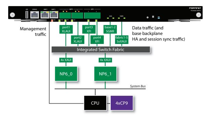
You can use the following get command to display the FortiGate-5001E NP6 configuration. The command output shows both NP6s connected to each interface with cross-chip offloading supported for all interfaces connected to the NP6 processors. You can also use the diagnose npu np6 port-list command to display this information.
