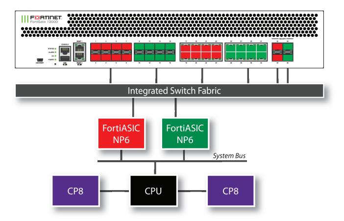
You can use the following get command to display the FortiGate 1200D NP6 configuration. The command output shows two NP6s named NP6\_0 and NP6\_1. The output also shows the interfaces (ports) connected to each NP6. You can also use the diagnose npu np6 port-list command to display this information.
