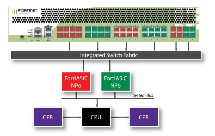
You can use the following get command to display the FortiGate 1500D NP6 configuration. The command output shows two NP6s named NP6\_0 and NP6\_1. The output also shows the interfaces (ports) connected to each NP6. You can also use the diagnose npu np6 port-list command to display this information.
