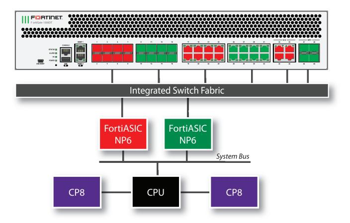
You can use the following get command to display the FortiGate 1500DT NP6 configuration. The command output shows two NP6s named NP6\_0 and NP6\_1. The output also shows the interfaces (ports) connected to each NP6. You can also use the diagnose npu np6 port-list command to display this information.
