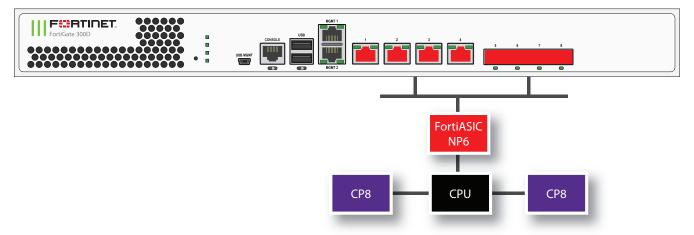
You can use the following get command to display the FortiGate 300D NP6 configuration. The command output shows one NP6 named NP6\_0 and the interfaces (ports) connected to it. You can also use the diagnose npu np6 port-list command to display this information.
