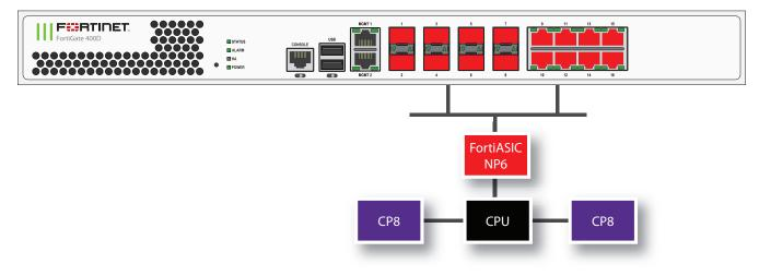
You can use the following get command to display the FortiGate 400D NP6 configuration. The command output shows one NP6 named NP6\_0 and the interfaces (ports) connected to it. You can also use the diagnose npu np6 port-list command to display this information.
