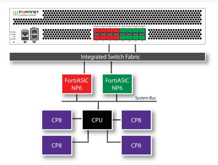
You can use the following get command to display the FortiGate 3000D NP6 configuration. The command output shows two NP6s named NP6\_0 and NP6\_1 and the interfaces (ports) connected to each NP6. You can also use the diagnose npu np6 port-list command to display this information.
