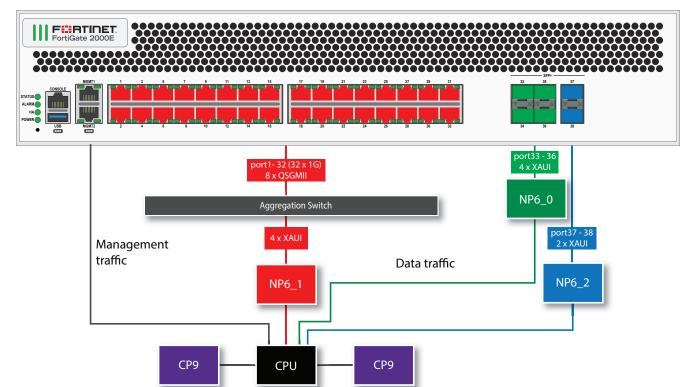
All data traffic passes from the data interfaces to the NP6 processors. Data traffic processed by the CPU takes a dedicated data path through the ISF and an NP6 processor to the CPU.
