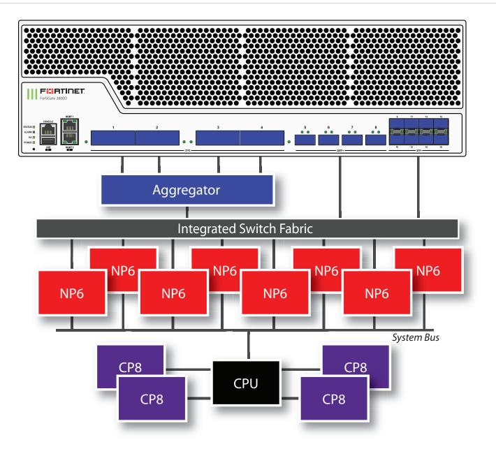
You can use the following get command to display the FortiGate 3800D NP6 configuration. The command output shows all NP6s connected to each interface (port) with cross-chip offloading supported for each port. You can also use the diagnose npu np6 port-list command to display this information.
