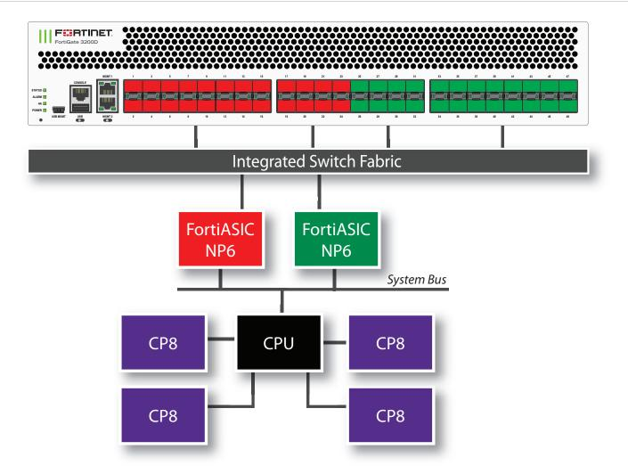
You can use the following get command to display the FortiGate 3200D NP6 configuration. The command output shows two NP6s named NP6\_0 and NP6\_1 and the interfaces (ports) connected to each NP6. You can also use the diagnose npu np6 port-list command to display this information.
