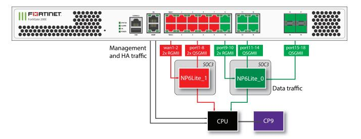
All data traffic passes from the data interfaces through to the NP6Lite processors. Data traffic to be processed by the CPU takes a dedicated data path through the ISF and an NP6Lite processor to the CPU.
