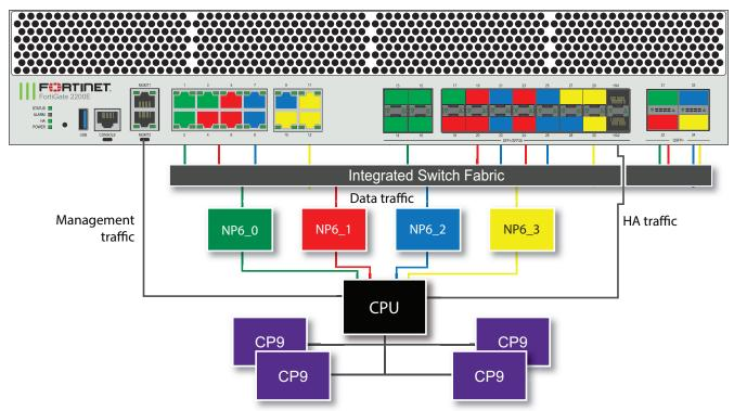
You can use the following command to display the FortiGate 2200E or 2201E NP6 configuration. The command output shows four NP6s named NP6\_0, NP6\_1, and NP6\_2 and the interfaces (ports) connected to each NP6. This interface to NP6 mapping is also shown in the diagram above.
