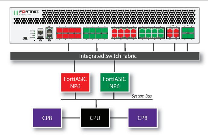
You can use the following get command to display the FortiGate 1500DT NP6 configuration. The command output shows two NP6s named NP6 $\_$ 0 and NP6 $\_$ 1. The output also shows the interfaces (ports) connected to each NP6. You can also use the <code>diagnose npu np6 port-list</code> command to display this information.
