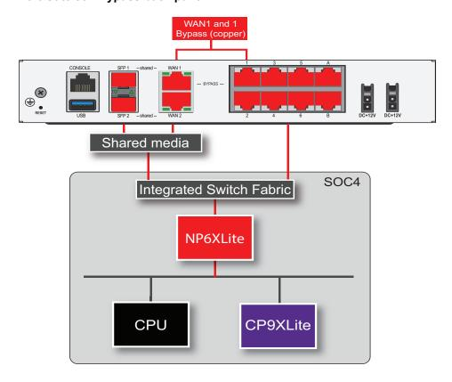
The SOC4 includes an integrated switch fabric (ISF) that connects all of the front panel network interfaces to the NP6XLite processor. The SOC4 ISF allows sessions passing between any FortiGate front panel interface pair to be offloaded by the NP6XLite processor. The SOC4 ISF also allows you to use the command config system virtual-switch to create a virtual hardware switch that can include any front panel interface connected to the SOC4.
