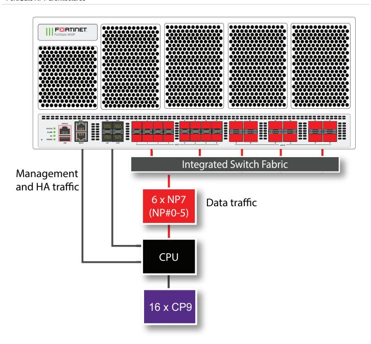
The FortiGate 4400F and 4401F each include six NP7 processors. All front panel data interfaces and the NP7 processors connect to the integrated switch fabric (ISF). All data traffic passes from the data interfaces through the ISF to the NP7 processors. All supported traffic passing between any two data interfaces can be offloaded by the NP7 processors. Data traffic processed by the CPU takes a dedicated data path through the ISF and an NP7 processor to the CPU.
