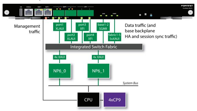
You can use the following get command to display the FortiGate-5001E NP6 configuration. The command output shows both NP6s connected to each interface with cross-chip offloading supported for all interfaces connected to the NP6 processors. You can also use the <code>diagnose npu np6 port-list</code> command to display this information.
