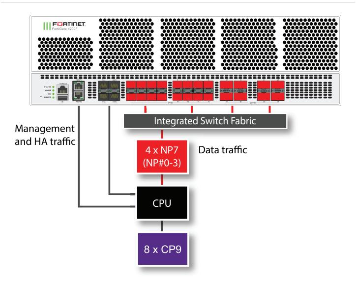
The FortiGate 4200F and 4201F each include four NP7 processors. All front panel data interfaces and the NP7 processors connect to the integrated switch fabric (ISF). All data traffic passes from the data interfaces through the ISF to the NP7 processors. All supported traffic passing between any two data interfaces can be offloaded by the NP7 processors. Data traffic processed by the CPU takes a dedicated data path through the ISF and an NP7 processor to the CPU.
