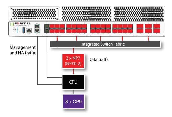
The FortiGate 3500F and 3501F each include three NP7 processors. All front panel data interfaces and the NP7 processors connect to the integrated switch fabric (ISF). All data traffic passes from the data interfaces through the ISF to the NP7 processors. All supported traffic passing between any two data interfaces can be offloaded by the NP7 processors. Data traffic processed by the CPU takes a dedicated data path through the ISF and an NP7 processor to the CPU.
