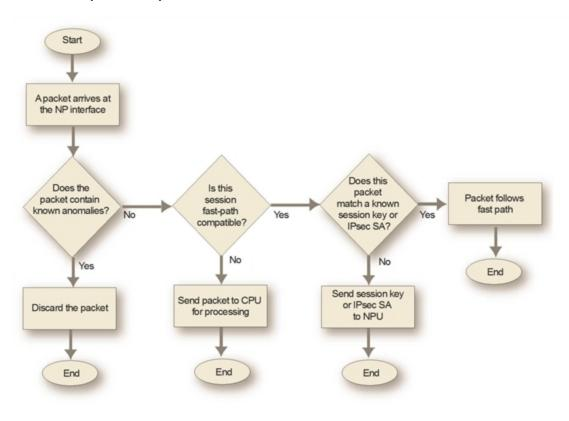
• If a matching session key or SA is not found, or if the packet does not meet packet requirements, the packet cannot be offloaded. The network processor sends the data to the FortiGate unit's CPU, which processes the packet.
