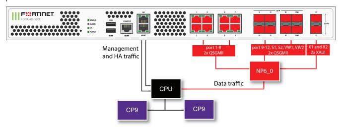
The FortiGate 500E and 501E each include one NP6 processor. All supported traffic passing between any two data interfaces can be offloaded by the NP6 processor. Data traffic to be processed by the CPU takes a dedicated data path through the NP6 processor to the CPU.
