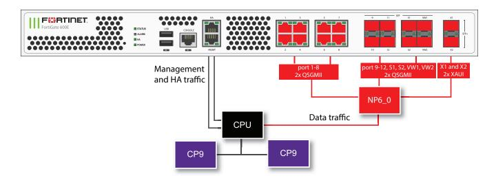
The FortiGate 600E and 601E each include one NP6 processor. All supported traffic passing between any two data interfaces can be offloaded by the NP6 processor. Data traffic to be processed by the CPU takes a dedicated data path through the NP6 processor to the CPU.
