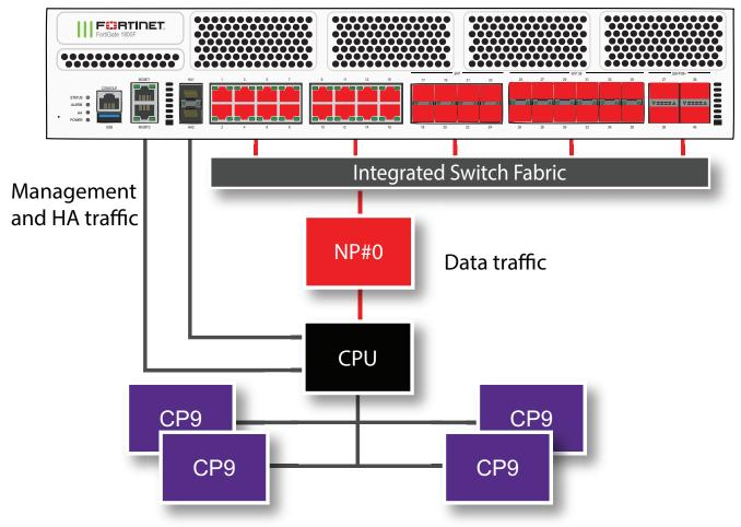
The FortiGate 1800F and 1801F each include one NP7 processor. All front panel data interfaces and the NP7 processor connect to the integrated switch fabric (ISF). All data traffic passes from the data interfaces through the ISF to the NP7 processor. All supported traffic passing between any two data interfaces can be offloaded by the NP7 processor. Data traffic processed by the CPU takes a dedicated data path through the ISF and the NP7 processor to the CPU.
