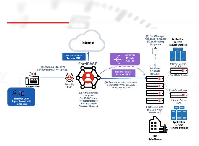
FortiSASE PoPs and the organization's FortiGate hubs form a traditional hub-and-spoke topology that supports the Fortinet autodiscovery VPN (ADVPN) configuration. ADVPN is an IPsec technology that allows a traditional hub-and-spoke VPN's spokes to establish dynamic, on-demand, direct tunnels, known as shortcut tunnels, between each other to avoid routing through the topology's hub device.
