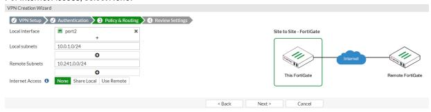
**5.** Proceed to create the VPN connection. After configuration, the VPN should automatically come up, and traffic can transverse. In the IBM Cloud console, you should see that the VPN gateway status is active and up.
