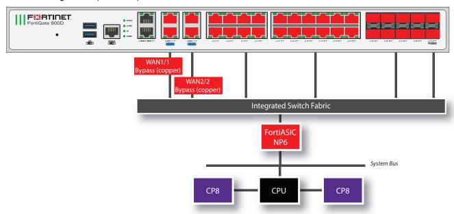
You can use the following get command to display the FortiGate 800D NP6 configuration. The command output shows one NP6 named NP6\_0. The output also shows all of the FortiGate 800D interfaces (ports) connected to NP6\_0. You can also use the diagnose npu np6 port-list command to display this information.
