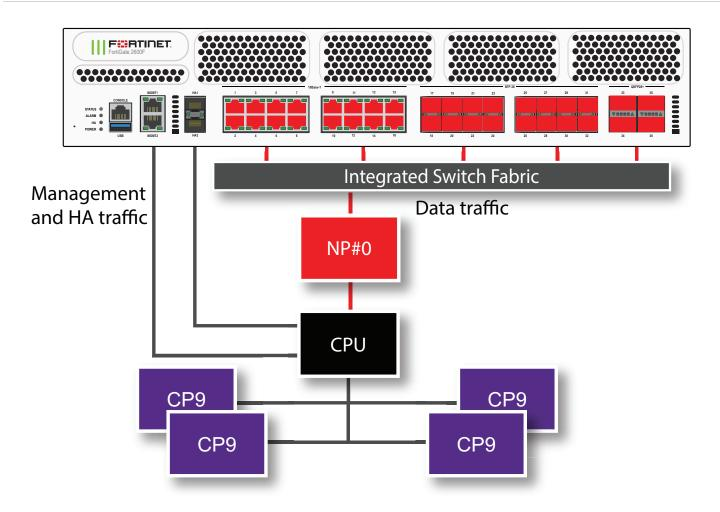
The FortiGate 2600F and 2601F each include one NP7 processor. All front panel data interfaces and the NP7 processor connect to the integrated switch fabric (ISF). All data traffic passes from the data interfaces through the ISF to the NP7 processor. All supported traffic passing between any two data interfaces can be offloaded by the NP7 processor. Data traffic processed by the CPU takes a dedicated data path through the ISF and the NP7 processor to the CPU.
