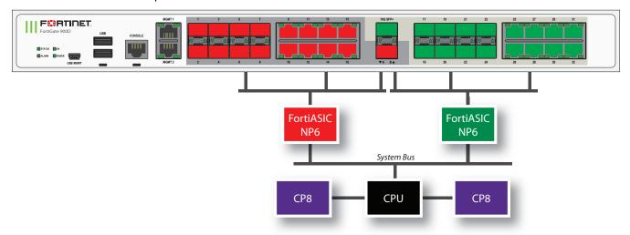
You can use the following get command to display the FortiGate 900D NP6 configuration. The command output shows two NP6s named NP6\_0 and NP6\_1. The output also shows the interfaces (ports) connected to each NP6. You can also use the diagnose npu np6 port-list command to display this information.
