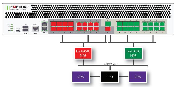
You can use the following get command to display the FortiGate 1000D NP6 configuration. The command output shows two NP6s named NP6\_0 and NP6\_1. The output also shows the interfaces (ports) connected to each NP6. You can also use the diagnose <code>npu np6 port-list</code> command to display this information.
