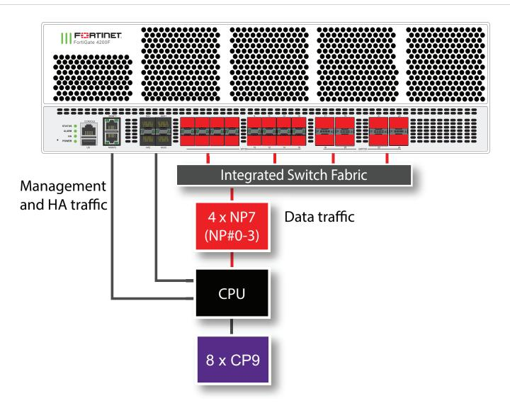
The FortiGate 4200F and 4201F each include four NP7 processors. All front panel data interfaces and the NP7 processors connect to the integrated switch fabric (ISF). All data traffic passes from the data interfaces through the ISF to the NP7 processors. All supported traffic passing between any two data interfaces can be offloaded by the NP7 processors. Data traffic processed by the CPU takes a dedicated data path through the ISF and an NP7 processor to the CPU.
