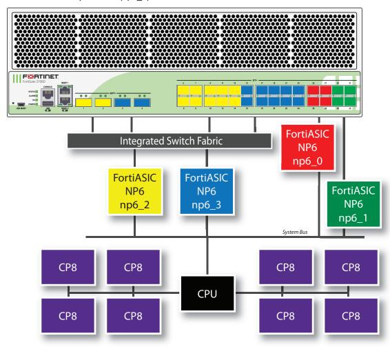
You can use the following get command to display the FortiGate 3700D NP6 configuration. In this output example, the first two NP6s (np6\_0 and np6\_1) are configured for low latency. The command output shows four NP6s named NP6\_0, NP6\_1, NP6\_2, and NP6\_3 and the interfaces (ports) connected to each NP6. You can also use the diagnose npu np6 port-list command to display this information.
