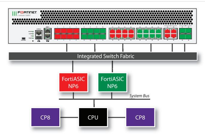
You can use the following get command to display the FortiGate 1500DT NP6 configuration. The command output shows two NP6s named NP6\_0 and NP6\_1. The output also shows the interfaces (ports) connected to each NP6. You can also use the diagnose npu np6 port-list command to display this information.
