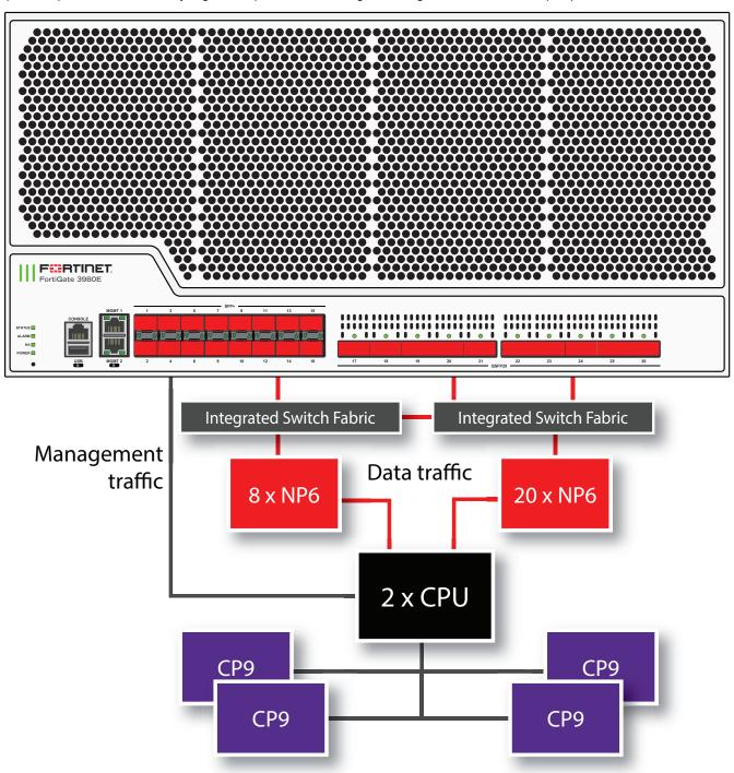
The FortiGate 3980E includes twenty-eight NP6 processors (NP6\_0 to NP6\_27). All front panel data interfaces and all of the NP6 processors connect to the integrated switch fabric (ISF). All data traffic passes from the data interfaces through the ISF to the NP6 processors.
