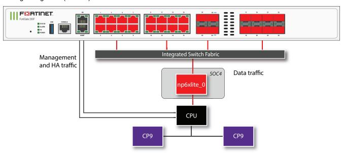
All front panel data interfaces and the NP6XLite processor connect to the integrated switch fabric (ISF). All data traffic passes from the data interfaces through the ISF to the NP6XLite processor. All supported traffic passing between any
