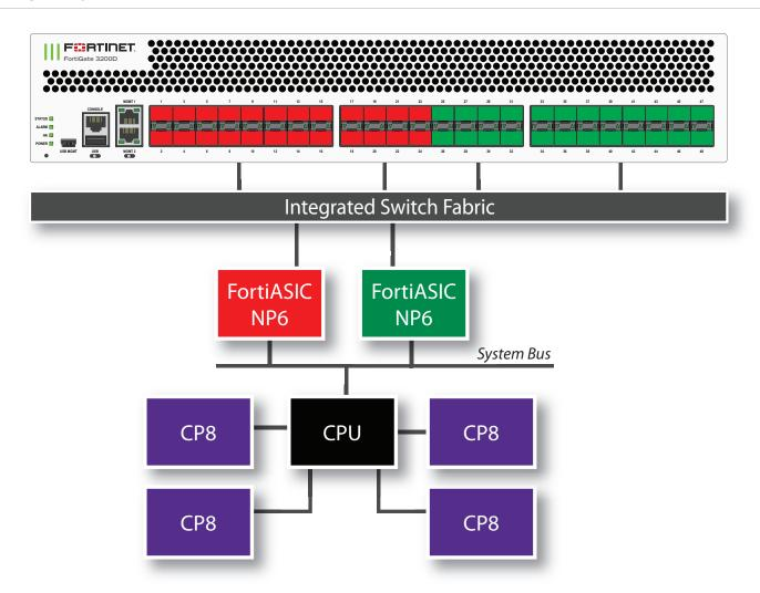
The FortiGate 3200D supports enhanced load balancing for LAG interfaces, see Enhanced load balancing for LAG interfaces for NP6 platforms on page 135.
