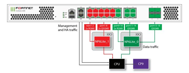
You can use the following get command to display the FortiGate 200E or 201E NP6Lite configuration. You can also use the diagnose npu np6lite port-list command to display this information.
