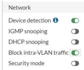
3. After you enable *Block Intra-VLAN traffic* in the example topology, packets sent from the hosts in VLAN40 are received by the VLAN40 interface of the FortiGate device and forwarded back to same interface. You need to use the FortiGate CLI to prevent traffic with the same local ingress and egress interface from being forwarded without a policy check:
