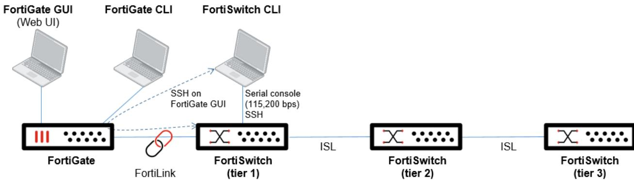
You can use the FortiGate GUI for most of the configurations. However, some features (such as routing offload and renaming FortiSwitch units) are only supported on the FortiGate CLI with FortiOS 7.4.3 and FortiSwitchOS 7.4.3.
