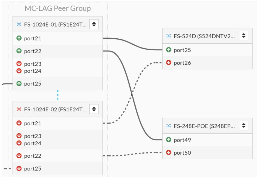
Enter the `diagnose switch mclag icl` command in the FortiSwitch CLI to see a detailed status of the ICL and split-brain detection.
