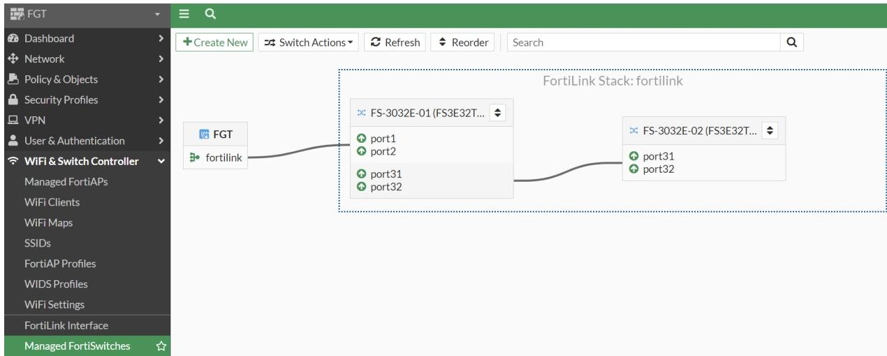
6. You can use the FortiGate GUI or CLI to configure an MCLAG on the Tier-1 FortiSwitch units. In the FortiGate GUI, hover the cursor over the link between the two FS-3032E switches to display the detail window:
