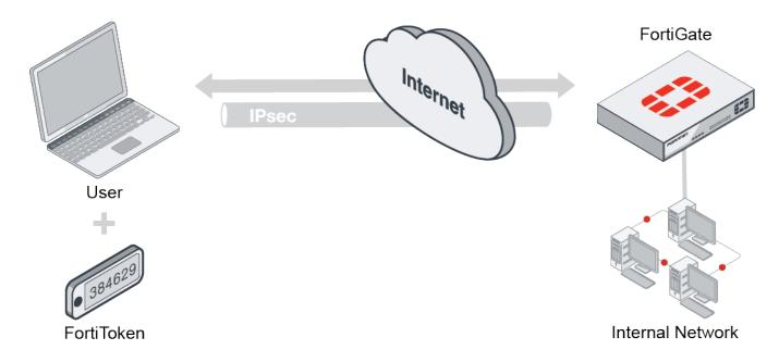
In this scenario, you will configure two-factor authentication using a FortiToken-200 for IPsec VPN connections.
