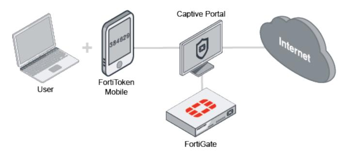
In this scenario, you will set up a FortiGate to require users on an internal network to use two-factor authentication with FortiToken Mobile to access the Internet through a captive portal.
