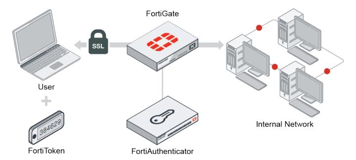
In this scenario, you will set up FortiAuthenticator to function as a RADIUS server to allow SSL VPN users to authenticate with a FortiToken-200.
