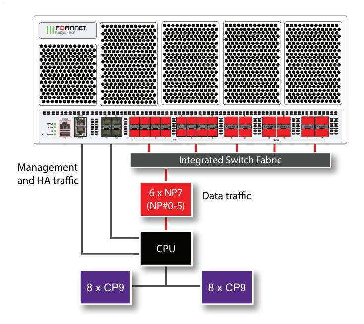
The FortiGate 4400F and 4401F each include six NP7 processors. All front panel data interfaces and the NP7 processors connect to the integrated switch fabric (ISF). All data traffic passes from the data interfaces through the ISF to the NP7 processors. All supported traffic passing between any two data interfaces can be offloaded by the NP7 processors. Data traffic processed by the CPU takes a dedicated data path through the ISF and an NP7 processor to the CPU.
