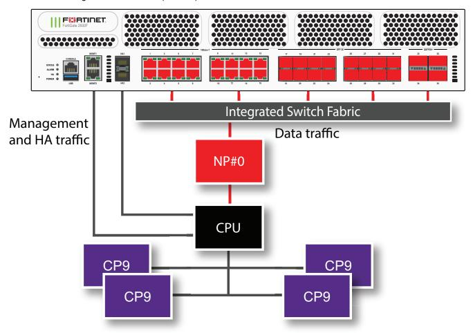
The FortiGate 2600F and 2601F each include one NP7 processor. All front panel data interfaces and the NP7 processor connect to the integrated switch fabric (ISF). All data traffic passes from the data interfaces through the ISF to the NP7
