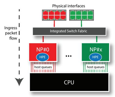
• The FortiGate-3600E has six NP6 processors and each NP6 processor has 20 host queues. All front panel data interfaces are connected to all NP6 processors over the integrated switch fabric. The default tcpsyn-ack-max setting of 600000 limits the of total number of TCP SYN\_ACK host packets per second that the FortiGate-3600E can process to 600000 x 20 x 6 = 72,000,000 TCP SYN\_ACK host packets per second.
