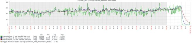
Using the system resources specified in the "Environment" and "Pre-Test Conditions" sections, it was observed that while the "Sustenance Test" was running the CPU utilization was normal and the performance of the system did not get impacted.
