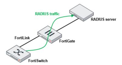
To control network access, you can configure 802.1x authentication from a FortiGate unit managing FortiSwitch units. A supplicant connected to a port on the switch must be authenticated by a RADIUS/Diameter server to gain access to the network.
