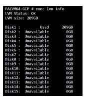
14. Run exec lvm extend. This incorporates the disk into the FortiAnalyzer system.
