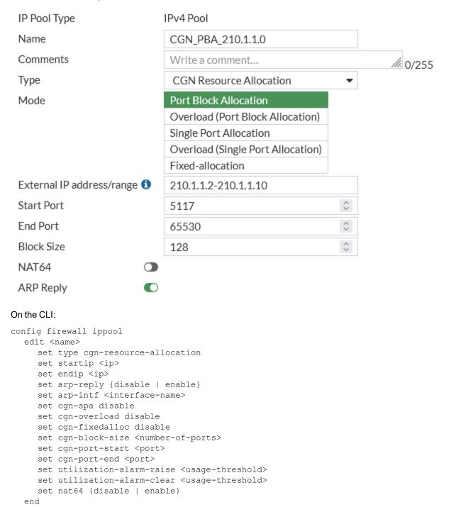
Port block allocation (PBA) reduces CGNAT logging overhead by creating a log entry only when a client first establishes a network connection and is assigned a port block. The number of log entries are reduced because a log entry is created when the port block is assigned, and not for each client connection.
