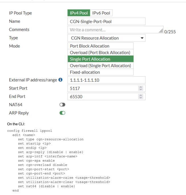
A single port allocation CGN resource allocation IP pool assigns single ports instead of ranges of ports. This type of CGN IP pool conserves ports by effectively reducing the port block size to 1. Since blocks of ports are not assigned to each client, this CGN IP Pool type works better for networks with large numbers of clients that start fewer individual sessions.
