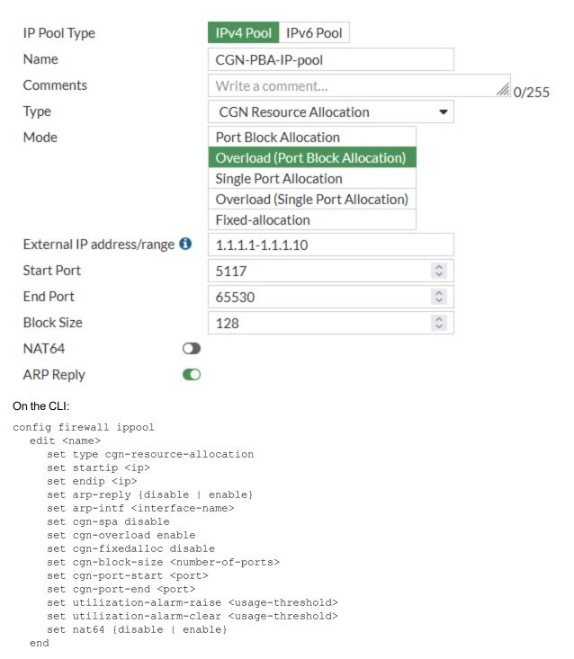
Overload with Port block allocation (PBA) reduces CGNAT logging overhead by creating a log entry only when a client first establishes a network connection and is assigned a port block. The number of log entries are reduced because a log entry is created when the port block is assigned, and not for each client connection. Overload causes FortiOS to re-use ports within a block, allowing for more possible connections before running out of ports.
