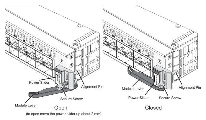
The FPM-7620F module levers align the module in the chassis slot and insert and eject the module from the slot. The power sliders activate micro switches that turn on or turn off power to the module. When both sliders are raised, the module cannot receive power. When the sliders are fully closed, the module can receive power if it is fully inserted into a chassis slot.
