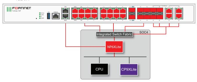
The SOC4 ISF also allows you to use the command <code>config system virtual-switch</code> to create a virtual hardware switch that can include any front panel interface connected to the SOC4.
