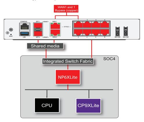
The SOC4 includes an integrated switch fabric (ISF) that connects all of the front panel network interfaces to the NP6XLite processor. The SOC4 ISF allows sessions passing between any FortiGate front panel interface pair to be offloaded by the NP6XLite processor. The SOC4 ISF also allows you to use the command <code>config system virtual-switch</code> to create a virtual hardware switch that can include any front panel interface connected to the SOC4.
