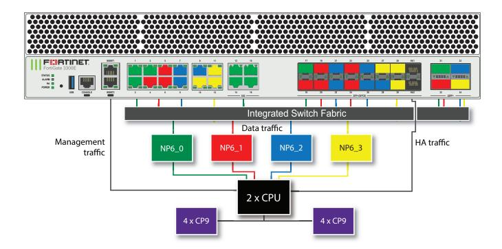
The FortiGate 3300E and 3301E each include four NP6 processors. All front panel data interfaces and all of the NP6 processors connect to the integrated switch fabric (ISF). All data traffic passes from the data interfaces through the ISF to the NP6 processors. Because of the ISF, all supported traffic passing between any two data interfaces can be offloaded by the NP6 processors. Data traffic processed by the CPU takes a dedicated data path through the ISF and an NP6 processor to the CPU.
