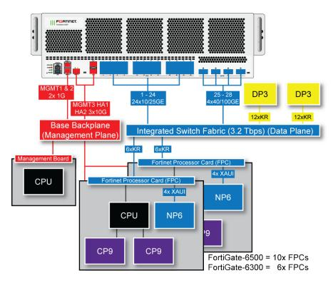
In the data plane, two DP3 load balancers use session-aware load balancing to distribute sessions from the front panel interfaces (port1 to 28) to Fortinet Processor Cards (FPCs). The DP3 processors communicate with the FPCs across the 3.2Tbps integrated switch fabric. Each FPC processes sessions load balanced to it. The FPCs send outgoing sessions back to the integrated switch fabric and then out the network interfaces to their destinations.
