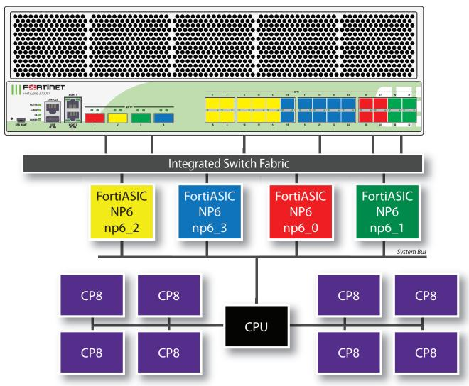
You can use the following get command to display the FortiGate 3700D NP6 configuration with low latency turned off for np6\_0 and np6\_1. The command output shows four NP6s named NP6\_0, NP6\_1, NP6\_2, and NP6\_3 and the interfaces (ports) connected to each NP6. You can also use the <code>diagnose npu np6 port-list</code> command to display this information.
