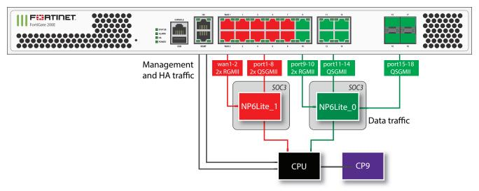
You can use the following get command to display the FortiGate 200E or 201E NP6Lite configuration. You can also use the diagnose <code>npu np6lite port-list</code> command to display this information.
