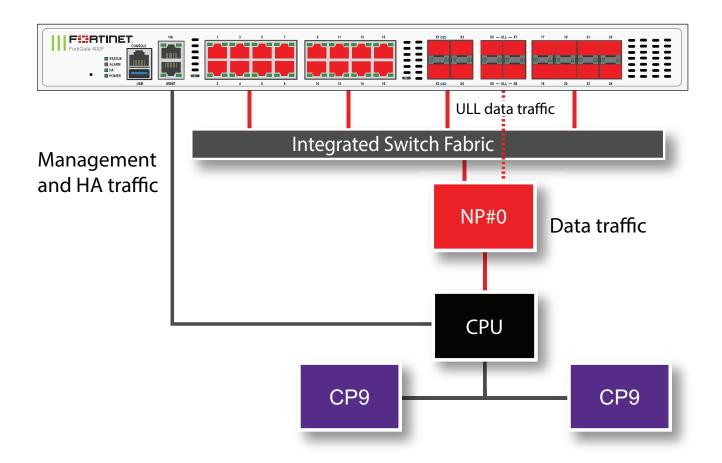
The MGMT interface is not connected to the NP7 processor. Management traffic passes to the CPU over a dedicated management path that is separate from the data path.
