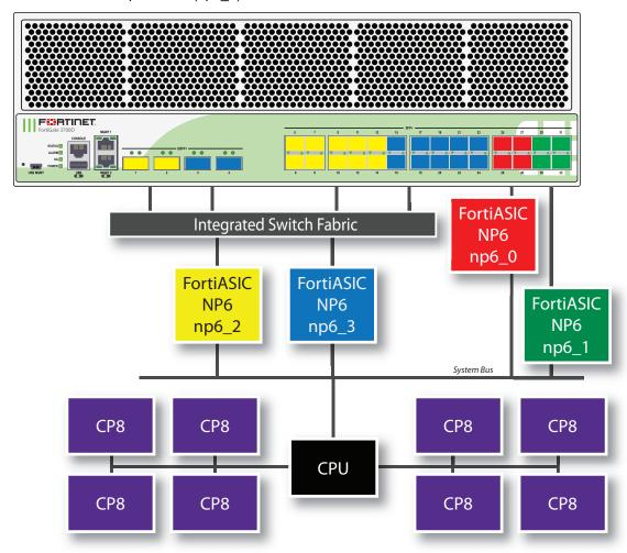
You can use the following get command to display the FortiGate 3700D NP6 configuration. In this output example, the first two NP6s (np6\_0 and np6\_1) are configured for low latency. The command output shows four NP6s named NP6\_0, NP6\_1, NP6\_2, and NP6\_3 and the interfaces (ports) connected to each NP6. You can also use the diagnose npu np6 port-list command to display this information.
