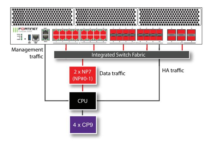
The FortiGate 3000F and 3001F each include two NP7 processors. All front panel data interfaces and the NP7 processors connect to the integrated switch fabric (ISF). All data traffic passes from the data interfaces through the ISF to the NP7 processors. All supported traffic passing between any two data interfaces can be offloaded by the NP7 processors. Data traffic processed by the CPU takes a dedicated data path through the ISF and an NP7 processor to the CPU.
