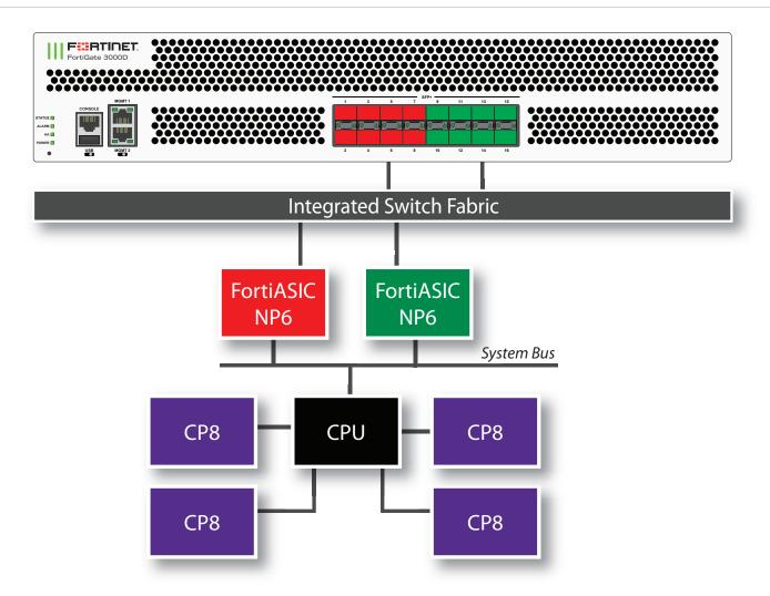
The FortiGate 3000D supports enhanced load balancing for LAG interfaces, see Enhanced load balancing for LAG interfaces for NP6 platforms on page 162.
