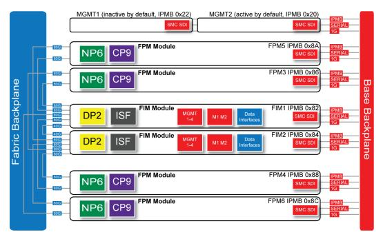
By default, MGMT2 is the active management module and MGMT1 is inactive. The active management module always has the Intelligent Platform Management Bus (IPMB) address 0x20 and the inactive management module always has the IPMB address 0x22.
