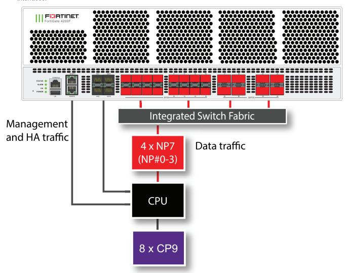
The FortiGate 4200F and 4201F each include four NP7 processors. All front panel data interfaces and the NP7 processors connect to the integrated switch fabric (ISF). All data traffic passes from the data interfaces through the ISF to the NP7 processors. All supported traffic passing between any two data interfaces can be offloaded by the NP7
