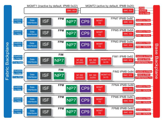
By default, MGMT2 is the active SMM and MGMT1 is inactive or passive. The active SMM always has the Intelligent Platform Management Bus (IPMB) address 0x20 and the passive SMM always has the IPMB address 0x22. Active and passive refers to the SMM that is controlling the chassis. The MGMT interfaces and console ports on both SMMs are always available.
