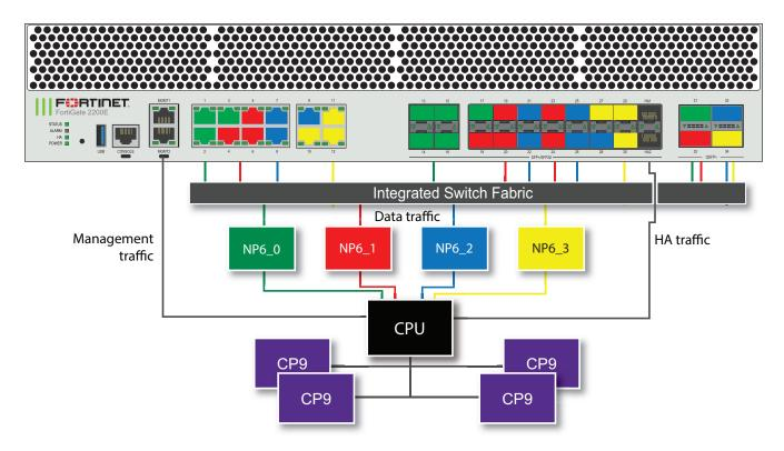
You can use the following command to display the FortiGate 2200E or 2201E NP6 configuration. The command output shows four NP6s named NP6\_0, NP6\_1, and NP6\_2 and the interfaces (ports) connected to each NP6. This interface to NP6 mapping is also shown in the diagram above.
