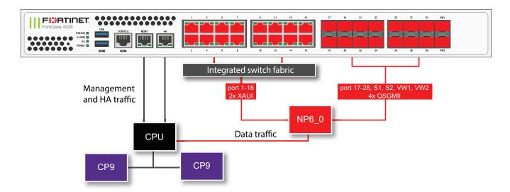
The FortiGate 400E and 401E each include one NP6 processor. All supported traffic passing between any two data interfaces can be offloaded by the NP6 processor. Data traffic to be processed by the CPU takes a dedicated data path through the NP6 processor to the CPU. Interfaces 1 to 16 connect to an integrated switch fabric to allow these sixteen interfaces to share two XAUI ports that connect to the NP6 processor.
