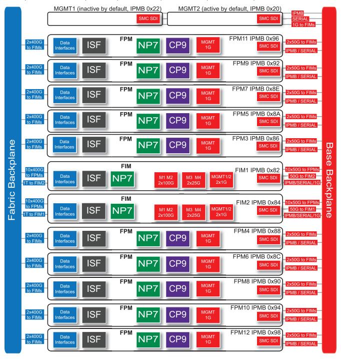
By default, MGMT2 is the active SMM and MGMT1 is inactive or passive. The active SMM always has the Intelligent Platform Management Bus (IPMB) address 0x20 and the passive SMM always has the IPMB address 0x22. Active and
