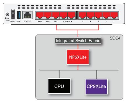
The SOC4 includes an integrated switch fabric (ISF) that connects all of the front panel network interfaces to the NP6XLite processor. The SOC4 ISF allows sessions passing between any FortiGate front panel interface pair to be offloaded by the NP6XLite processor. The SOC4 ISF also allows you to use the command config system virtual-switch to create a virtual hardware switch that can include any front panel interface connected to the SOC4.
