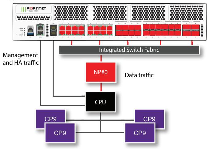
The MGMT interfaces are not connected to the NP7 processor. Management traffic passes to the CPU over a dedicated management path that is separate from the data path. You can also dedicate separate CPU resources for management traffic to further isolate management processing from data processing (see Improving GUI and CLI responsiveness (dedicated management CPU) on page 21).
