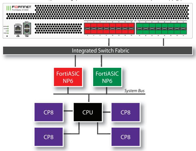
The FortiGate 3100D supports enhanced load balancing for LAG interfaces, see Enhanced load balancing for LAG interfaces for NP6 platforms on page 162.
