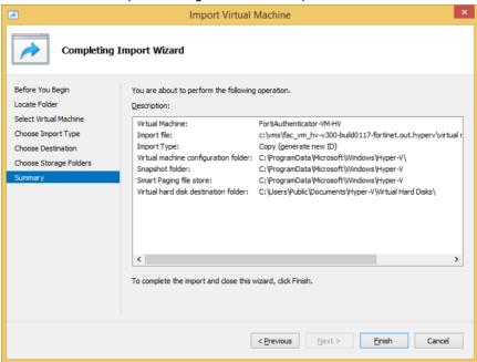
**9.** The VM will be installed and will be displayed in the Hyper-V Manager. Once complete, and before the VM is started, the hardware settings can be modified. Right-click the new VM and select *Settings...*.
