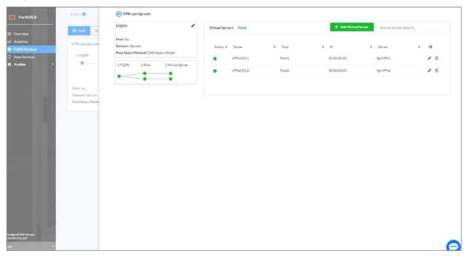
After completing these steps, the customer can monitor the VPN service status from both Location1 and Location2 on the FQDN service detail page. The FortiGSLB will load balance the traffic to the server that have the nearest location. If the nearest location VPN server is down, the FortiGSLB will direct the traffic to other available location. If both VPN service servers are not available, the FortiGSLB will direct traffic to the default VPN server.
