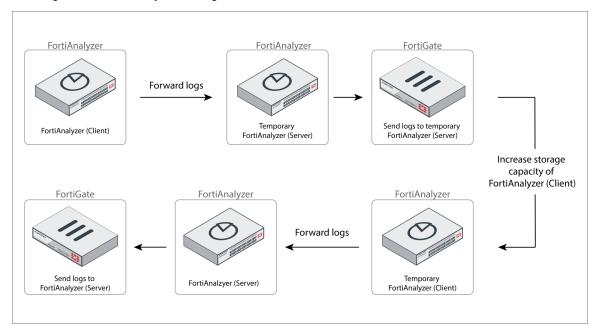
You can use this procedure when upgrading the default 12 HDD (hard disk drive) for FAZ-4000B or FAZ-3500E to the maximum 24 HDD.
