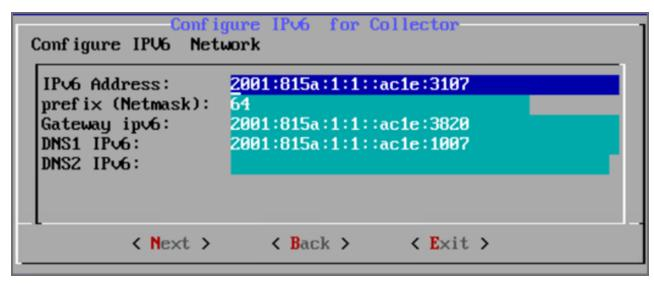
**Note**: If you chose option **3** in step 9 for both IPv4 and IPv6, then even if you configure 2 DNS servers for IPv4 and IPv6, the system will only use the first DNS server from IPv4 and the first DNS server from the IPv6 configuration. **Note**: In many dual stack networks, IPv4 DNS server(s) can resolve names to both IPv4 and IPv6. In such environments, if you do not have an IPv6 DNS server, then you can use public IPv6 DNS servers or use IPv4-mapped IPv6 address.
