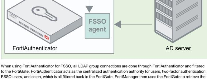
filter information from the CA server. When using this setup, it is recommended to position the FortiGate physically close to the CA server to keep latency low.
