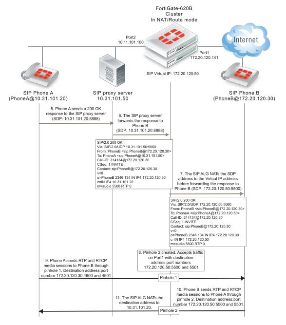
The media stream from Phone A is accepted by pinhole one and forwarded to Phone B. The source address of this media stream is changed to the SIP proxy server virtual IP address. The media stream from Phone B is accepted by pinhole 2 and forwarded to Phone B. The destination address of this media stream is changed to the IP address of Phone A.
