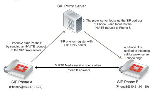
A common SIP configuration would include multiple networks of SIP phones. Each of the networks would have its own SIP server. Each SIP server would proxy the communication between phones on its own network and between phones in different networks.
