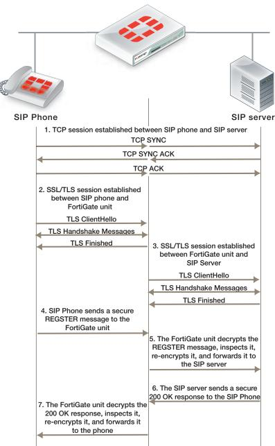
Other than enabling SSL mode and making sure the security policies accept the encrypted traffic, the FortiGate configuration for SSL/TLS SIP is the same as any SIP configuration. SIP over SSL/TLS is supported for all supported SIP configurations.
