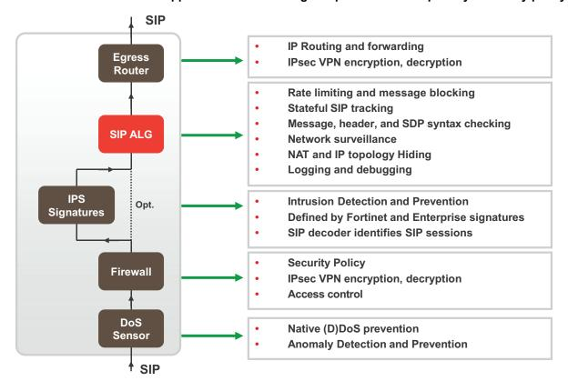
The SIP ALG works at the application level after ingress packets are accepted by a security policy
