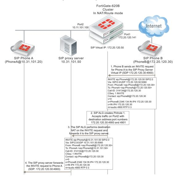
To simplify the diagrams, some SIP messages are not included (for example, the Ringing and ACK response messages) and some SIP header lines and SDP profile lines have been removed from the SIP messages.
