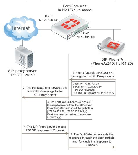
The more specific a pinhole is the more secure it is because it accept less traffic. In this situation, the pinhole would be more secure if it only accepted traffic from the SIP server. This is what happens if strict-register is enabled in the VoIP profile that accepts the REGISTER request from Phone A.
