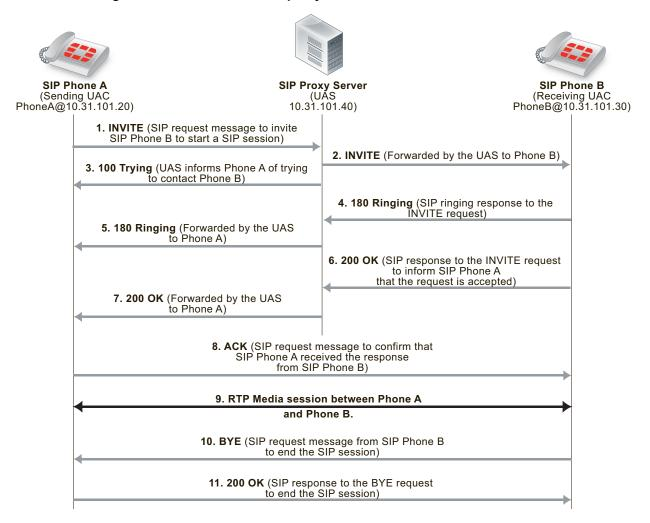
The SIP messages include SIP headers that contain names and addresses of Phone A, Phone B and the proxy server. This addressing information is used by the UACs and the proxy server during the call set up.
