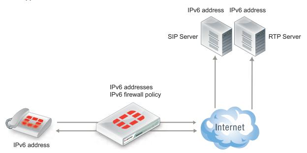
To enable SIP support for IPv6 add an IPv6 security policy that accepts SIP packets and includes a VoIP profile.
