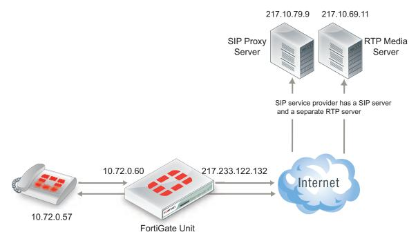
In the scenario, shown above, the SIP phone connects to a VIP (10.72.0.60). The SIP ALG translates the SIP contact header to 217.10.79.9, opens RTP pinholes, and manages NAT.
