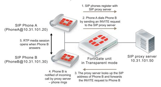
The phones and server use the same SIP dialogs as they would if the FortiGate was not present. However, the FortiGate can be configured to control which devices on the network can connect to the SIP proxy server and can also protect the SIP proxy server from SIP vulnerabilities.
