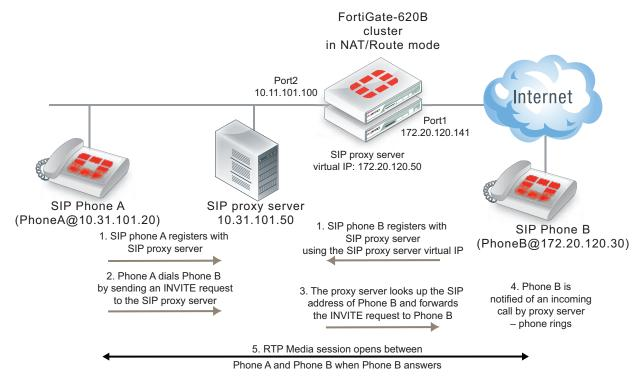
The phones and server use the same SIP dialog as they would if the FortiGate was not present. However, the FortiGate can be configured to control which devices on the network can connect to the SIP proxy server and can also protect the SIP proxy server from SIP vulnerabilities. In addition, the FortiGate has a firewall virtual IP that forwards packets sent to the SIP proxy server Internet IP address (172.20.120.50) to the SIP proxy server internal network IP address (10.31.101.30).
