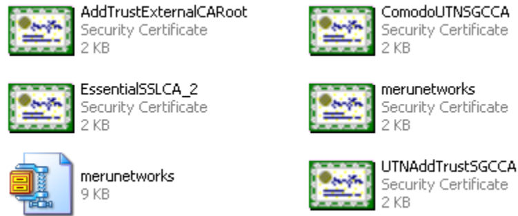
Figure 46: Sample Certificates Returned by CA (Server, Intermediate, and Root)
